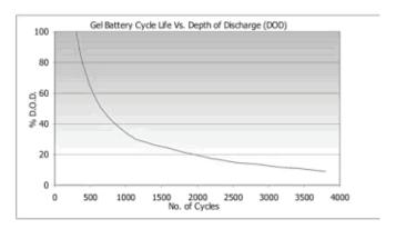
$\begin{array}{lll} \mbox{Nominal voltage} & 6 \& 12 \mbox{ volts} \\ \mbox{Design life} & 12 \mbox{ Years @ 20°C} \\ \mbox{Operating temperature} & -10 \mbox{ °C to } 50 \mbox{ °C} \\ \end{array}$
